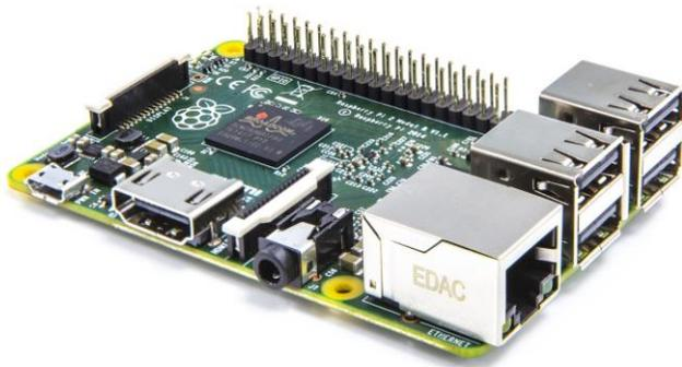
Fig. 11. Raspberry Pi 2 Model B [21].
